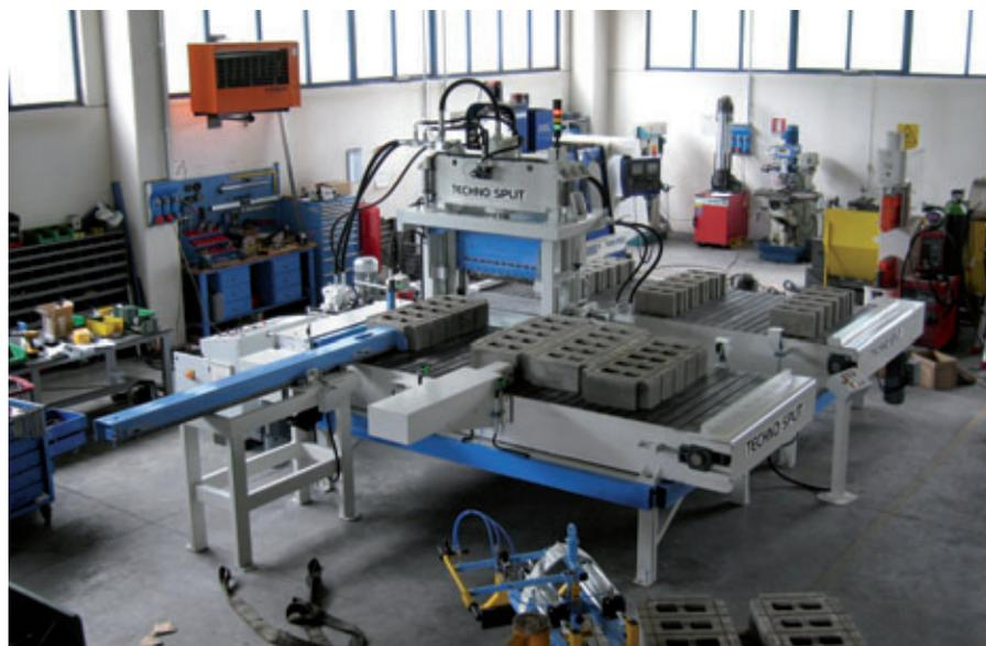
*The Dubai system features a splitting machine with a splitting length of 800 mm, 280 mm splitting height and 80 ton splitting force*
