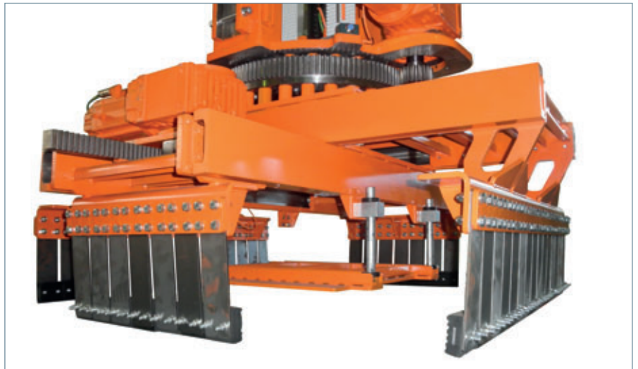
The new splitting system features an automatic gripper with electrical power clamping
